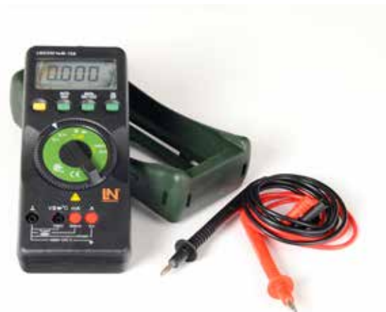
Multimeter with optical data interface for display via a virtual instrument on a PC
